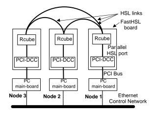
Figure 1. MPC architecture
