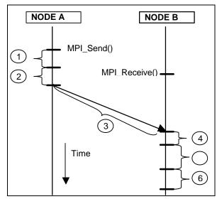
Figure 10. MPI task to task transfer schedule
