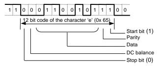
Figure 2. HSL 12 bits symbol coding
