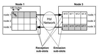
Figure 6. Memory slot structure
