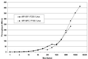
Figure 8. MPI-MPC and MPI-BIP throughput comparison
